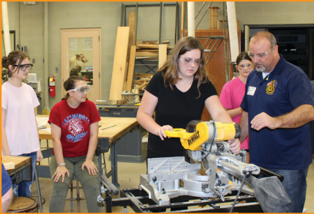
Skilled Tradesman Brian Beachy teaching students how to use a miter saw.
